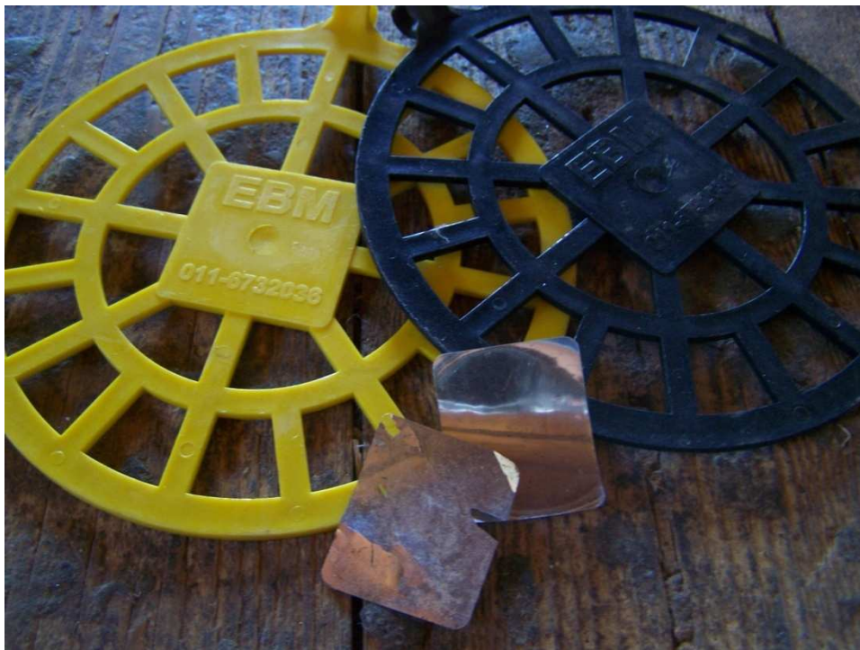
Fig. 2: The 'pods' installed in 2007. These 'pods' worked perfectly until the reflective pads fell off. Note that the reflective pads are small, but still proved effective.
